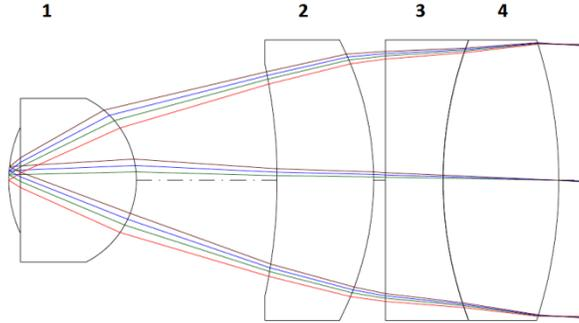
Fig. 2. Optical design of the miniature objective lens.
