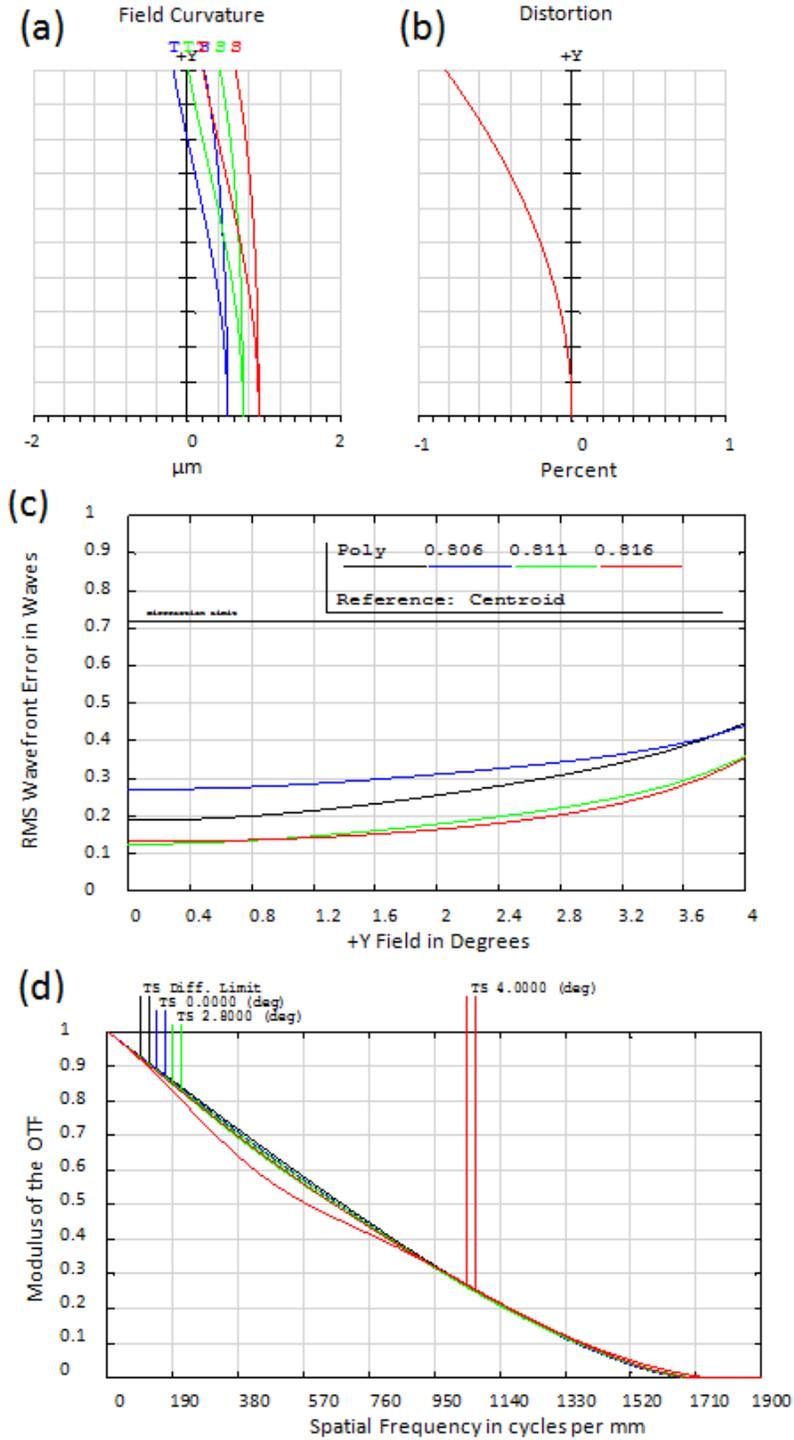
Fig. 3. (a) Field curvature and (b) distortion of the miniature objective lens design for wavelengths of 0.806  $\mu\text{m}$  (blue), 0.811  $\mu\text{m}$  (green), and 0.816  $\mu\text{m}$  (red). Maximum field is 4 degrees. (c) RMS wavefront error across field. (d) Polychromatic diffraction modulation transfer function of the miniature objective lens design for the fields above and for wavelengths from 0.806 to 0.816  $\mu\text{m}$ .
