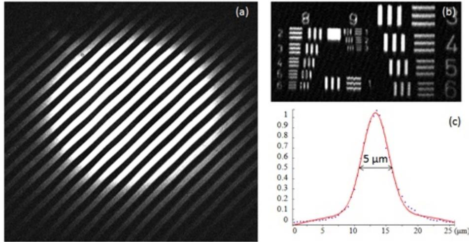
Fig.7. (a) Ronchi ruling showing 550  $\mu\text{m}$  FOV of the rCLE with miniature objective lens. (b) Groups 8, 9 and 7 (to the right) of USAF target at 0 mA ETL current. (c) Axial resolution plot showing a FWHM of 5  $\mu\text{m}$  at 0 mA ETL current.
